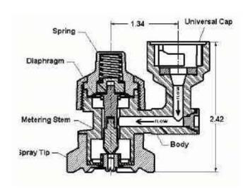
VariTarget is a nozzle that is capable of controlling flow rate and maintaining proper spray pattern and droplet size over an extended range of flow rates. The nozzle comprises a flexible spray tip that is automatically and appropriately deformed by a flexible metering assembly in response to changes in liquid pressure. Application rate from 5 to 40 GPA and spray speed from 5 to 25 MPH is achievable with one VariTarget nozzle.
