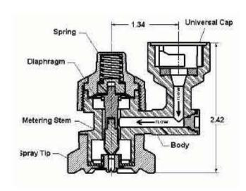
VariTarget is a nozzle that is capable of controlling flow rate and maintaining proper spray pattern and droplet size over an extended range of flow rates. The nozzle comprises a flexible spray tip that is automatically and appropriately deformed by a flexible metering assembly in response to changes in liquid pressure. Application rate from 3 to 30 GPA and spray speed from 4 to 20 MPH is achievable with one VariTarget nozzle (Orange Tip).
